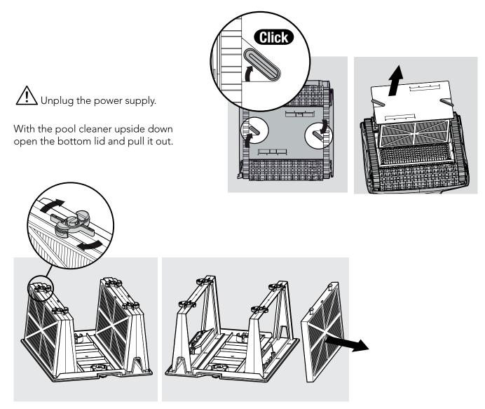
Open the clips and remove the filters.
