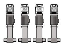
A second way of splitting (named COMBO) consists of using several pumps in parallel (up to 8) each driven by an inverter.
