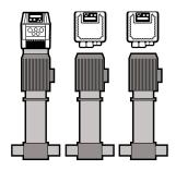
A first method of splitting consists of installing one pump driven by the inverter and 1 or 2 DOL pumps directly connected to the main power (Direct On Line). Inverter switches the 1 or 2 DOL pumps on/off through contactors. Inverter alternates the two DOL pumps to average pump wear.
