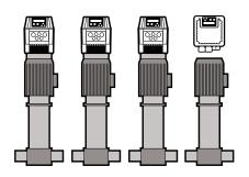
Additionally it is possible to equip the system with pumps connected in COMBO mode plus 1 or 2 DOL pumps to satisfy additional water demand.
