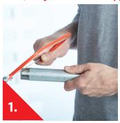
Roughen the thread with saw-blade or file
