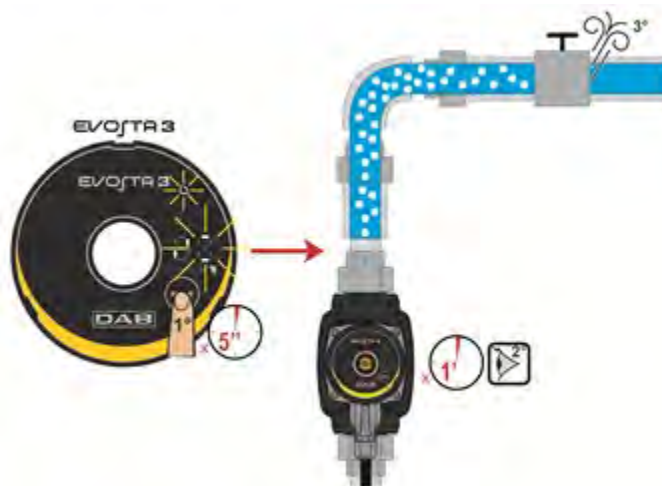
Figure 9: Automatic venting of the pump
