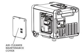
8.2.2)Loosen the air cleaner cover screws and remove the cover.
