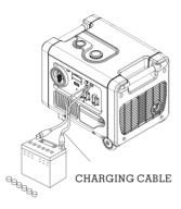
Do not start the automobile engine when the generator is still connected to the battery, otherwise the generator will be damaged.
