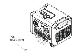
Tighten oil drain plug with 25-30 N.m
