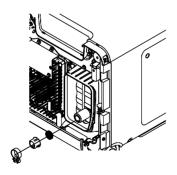
8.4.3)Use a brush to remove carbon deposits from the spark arrester. If the spark arrester is wear, replace it.
