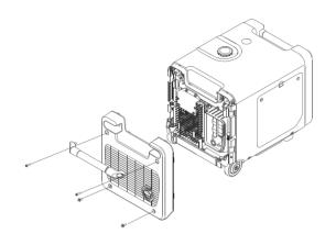
8.4.2) Take off the spark arrester from the muffler after the engine cool down.
