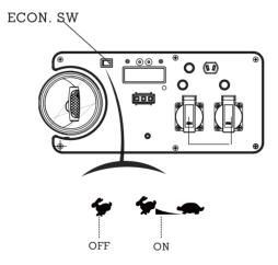
■ When a high load electrical appliance is connected instantaneously, in order to reduce voltage change, turn the economy control switch to the "OFF" (\*) position.
