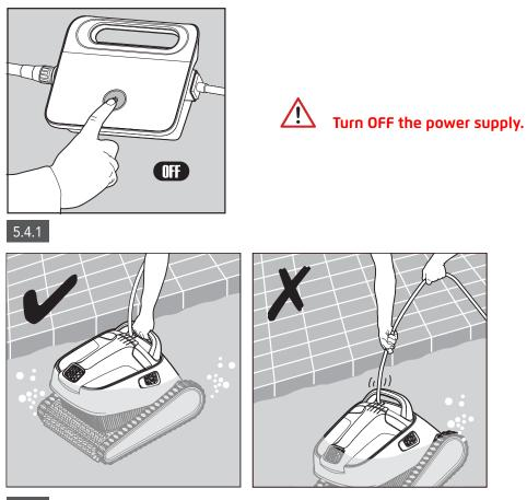
5.4.2 Using the blue cable, bring the Pool Cleaner to the pool edge. Use the handle to remove the Pool Cleaner from the pool.
