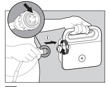
**5.1.3** Attach the blue cable to the power supply by inserting it with the notch on the connector (1) lined up to the groove in the socket on the power supply. Turn it clockwise (2).
