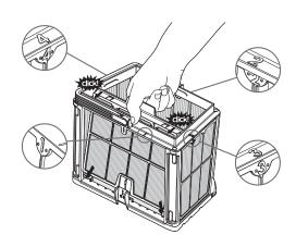
8.2.5 Reassemble the filter panels in the order  $4 \rightarrow 3 \rightarrow 2 \rightarrow 1.$
