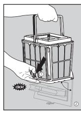
8.1.4 The debris can then be removed.
