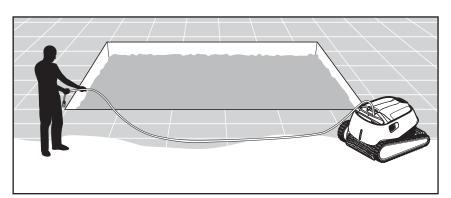
5.1.2 Unwind the blue cable and stretch it out completely so that it has no kinks.
