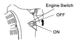
**NOTE:** Turn the engine switch to the OFF position immediately to shut down the engine in an emergency.
