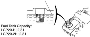
It is recommended to use fresh, unleaded gasoline with an octane rating of 90 or 93. Use of ethanol gasoline (more than 10% blended) is not allowed.
