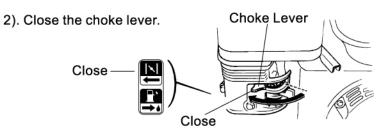
**NOTE:** In case the engine is warm or ambient temperature is high, it's not necessary to close the choke lever.
