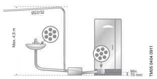
Fig. 41 Example of installation
