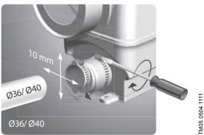
Fig. 25 Height and side alignment possible when using Ø36/40 inlet pipes
