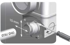
Fig. 35 Height and side alignment possible when using Ø36/40 inlet pipes
