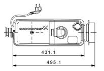
Fig. 27 Dimensional drawings, Sololift2 CWC-3
