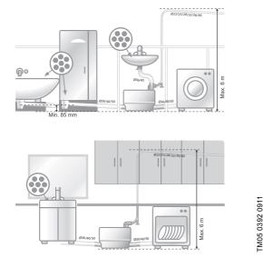
Fig. 31 Examples of installation
