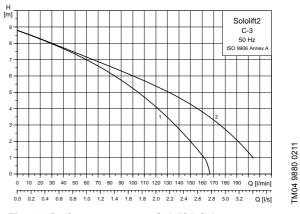
Fig. 36 Performance curves, Sololift2 C-3
