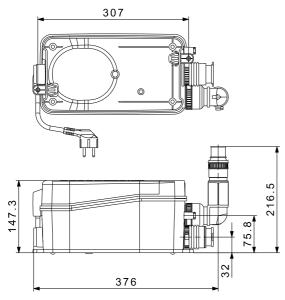
Fig. 44 Dimensional drawings, Sololift2 D-2
