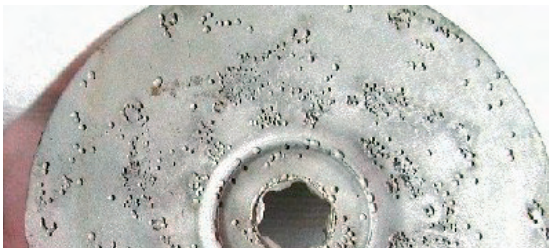
Pitting corrosion of EN 1.4401 (AISI 316)
