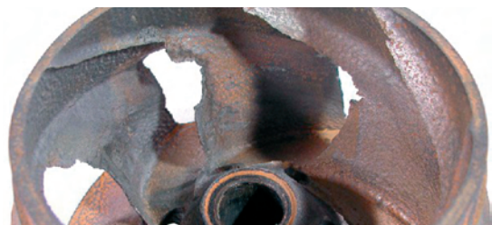
Erosion corrosion of cast iron impeller
