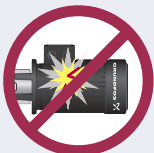
Fig 1.4.6: With non-sparking motors ExnA, no ignition is likely to occur.
