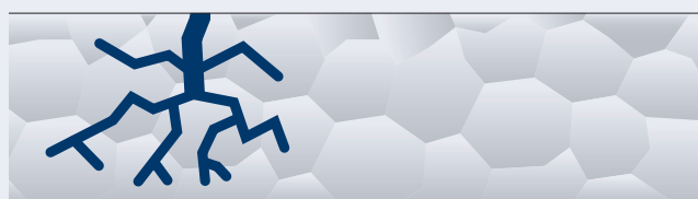
Fig. 1.6.10: Stress corrosion cracking
