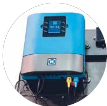
Control Station Touch Screen
